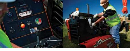
Experience built the Ditch Witch® JT5 Horizontal Directional Drill. With input from our customers and their many years of experience installing utilities on tight jobsites, our engineers developed the ideal compact rig with the right amount of thrust and pullback for shallow installations of cable, fiber and water systems up to 150 feet in length (46 m) beneath roads, driveways, sidewalks, sensitive landscaping, and other surface obstacles. The JT5 is a true team effort.
